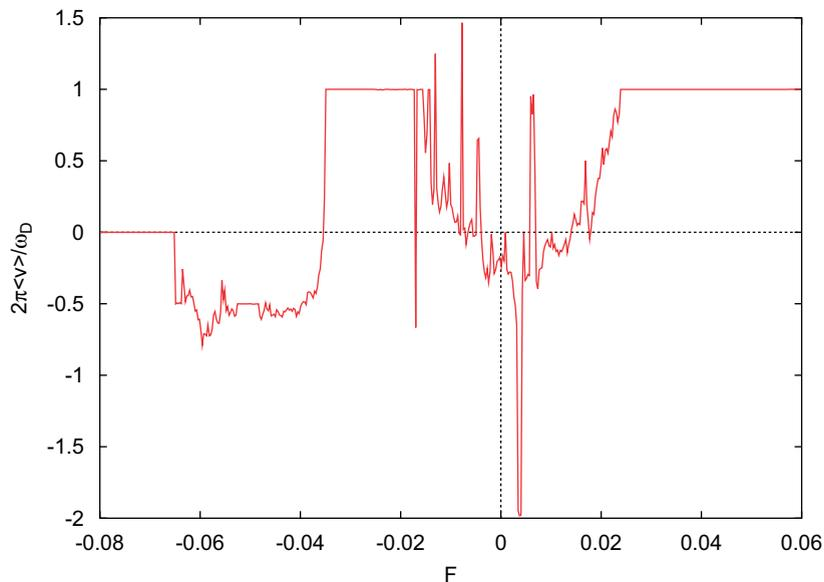
Fig. 3. The detailed structure of the scaled average velocity  $2\pi\langle v \rangle / \omega_D$  as a function of the amplitude of the external force  $F$ , around  $F = 0$ , for  $F_D = 1.0$  and  $\omega_D = 0.6$ . Notice the step at  $2\pi\langle v \rangle / \omega_D = 1$  in the interval  $-0.035 < F < -0.0175$ , indicating anomalous negative mobility.
